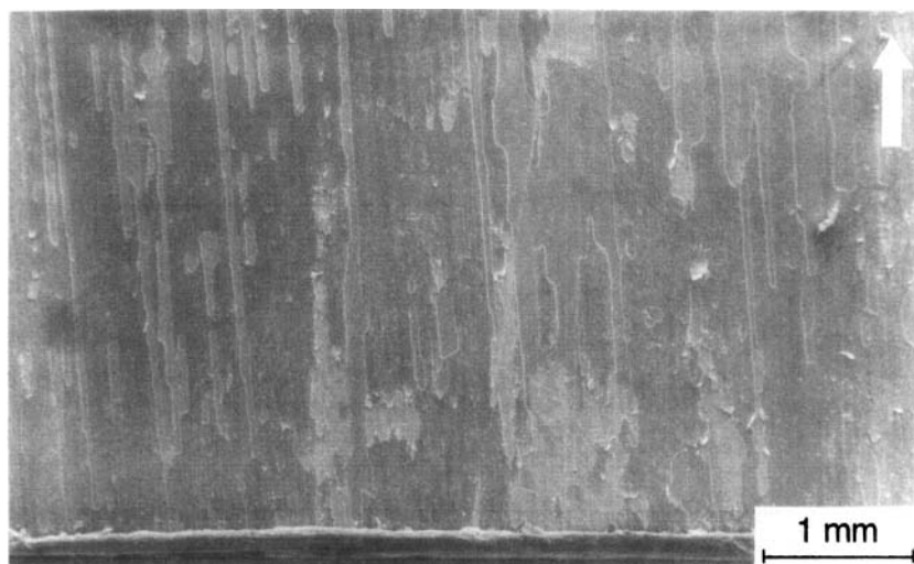
FIGURE 8 Fracture surface morphology of an adhesive joint with t = 0.02 mm. (Arrow indicates direction of crack propagation).
